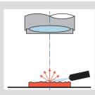
With incident illumination at an extremely flat angle, added contrast is produced by the high light yield and distinct shadows.
